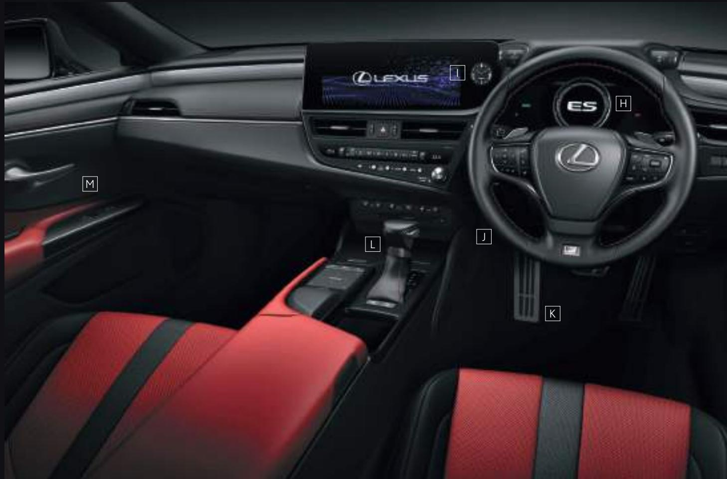
H\_Meters &amp; multi-information display / I\_Clock / J\_Steering wheel / K\_Aluminum pedals / L\_Shift lever knob / M\_Trim
