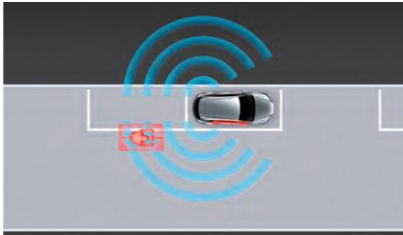
Advanced Park 6 functions - perpendicular parking (reverse) - perpendicular parking (forward) - perpendicular exiting (reverse) - perpendicular exiting (forward) - parallel parking - parallel exiting
