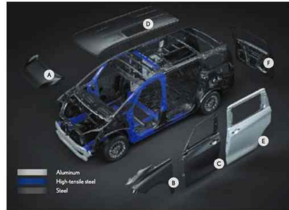
LM's chassis and body structures employ substantial bracing and reinforcement to maintain a calm, predictable driving composure. Overall rigidity is increased, drastically reducing yaw, pitch and roll. Added reinforcement is found at the front and rear suspension (structural support), radiator (front circular structure), cowl (steering system stiffener and bracing), and B-, C-, and D-pillars (gusset structures).
